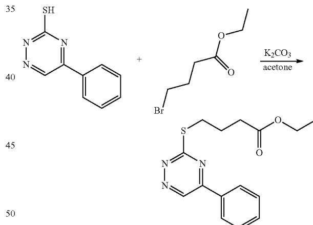
K<sub>2</sub>CO<sub>3</sub> (6.14 g, 0.044 mol) is added to a solution of 5-phenyl-1,2,4-triazine-3-thiol (8.412 g, 0.044 mol) in acetone (250 ml). The reaction medium is subsequently stirred for 15 minutes and 95% ethyl 4-bromobutyrate (9.13 g, 0.044 mol) is added dropwise. The reaction medium is brought to reflux for 2.5 hours and then the mixture is cooled down to 20°C. and filtered. The evaporation of the solvent under reduced pressure produces a black oil.
