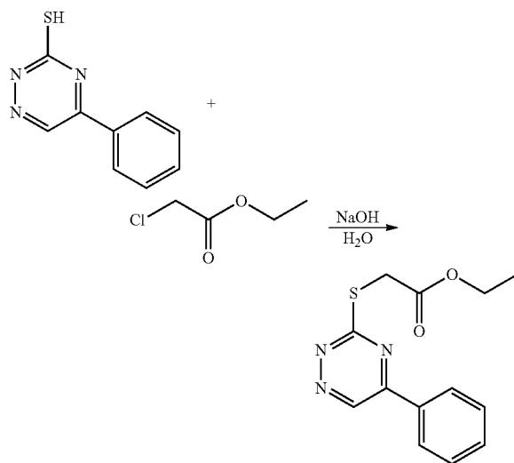
Ethyl chloroacetate (9.608 g, 0.078 mol) is added dropwise at ambient temperature to a solution of 5-phenyl-1,2,4-triazine-3-thiol (14.84 g, 0.078 mol) and sodium hydroxide (3.136 g, 0.078 mol) in 450 ml of water. The reaction medium is subsequently stirred vigorously for 2 hours and then filtered, and the filter residue is washed with water (2 l).
