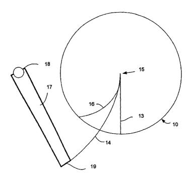
(57) **Abstract:** Hard disk servo data is recorded on a stamper master or a hard disk with a timing offset that converts the arc (14) described by the servo data writer's rotary actuator (17) into the arc described by the disk drive's rotary actuator.
