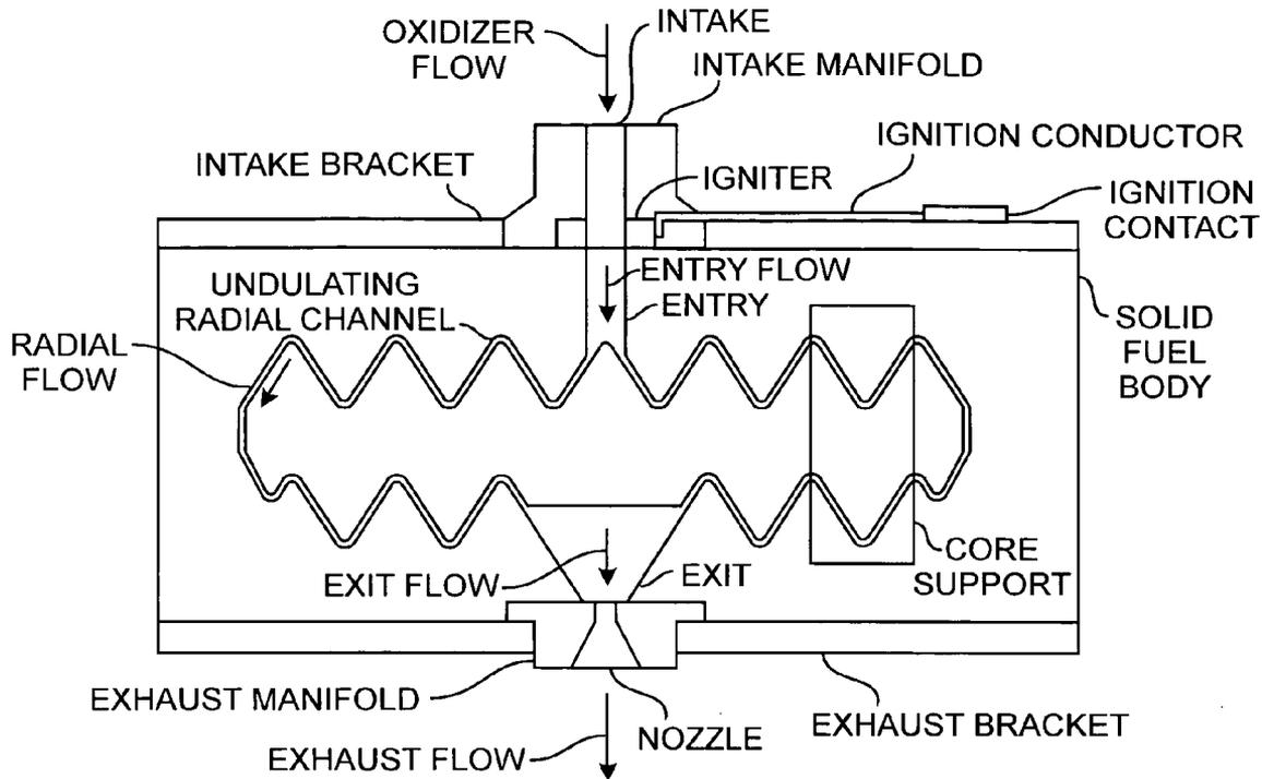
UNDULATING RADIAL CHANNEL SOLID FUEL STEREOLITHOGRAPHIC ROCKET MOTOR
