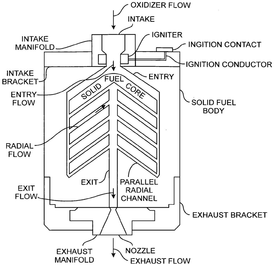
PARALLEL RADIAL CHANNEL SOLID FUEL STEREOLITHOGRAPHIC ROCKET MOTOR
