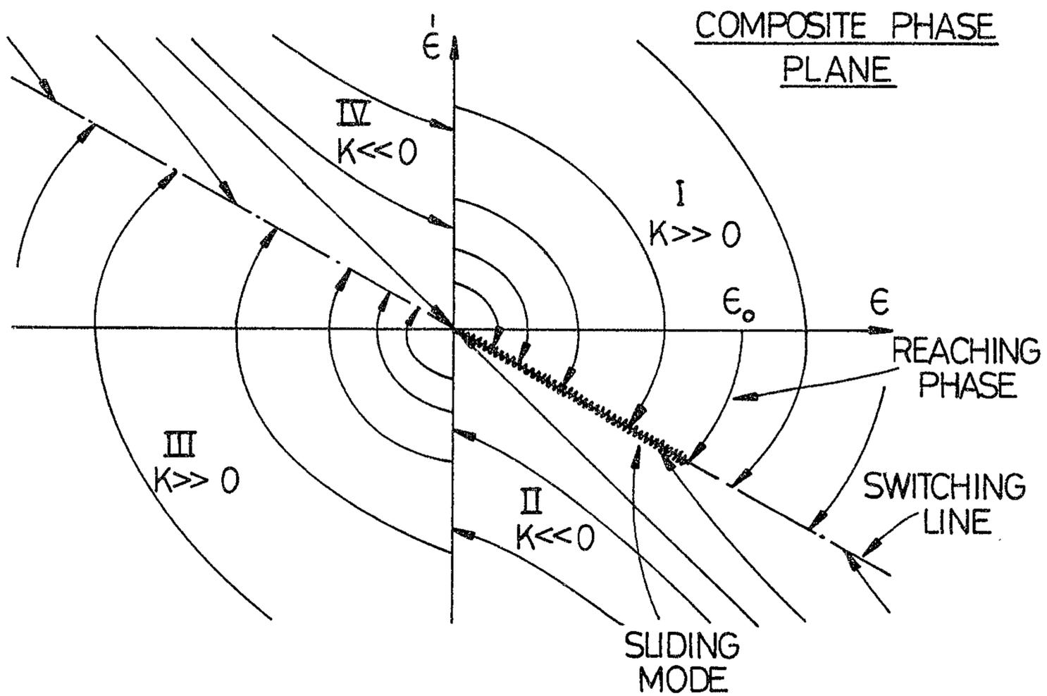
Fig. 5 COMPOSITE PHASE PLANE & TRANSIENT RESPONSE
