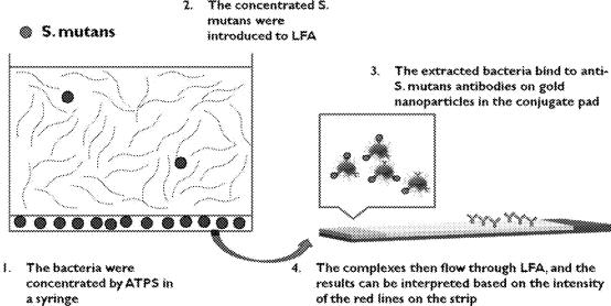
The entire assay is completed in 20 min (10 min ATPS + 10 min LFA)
