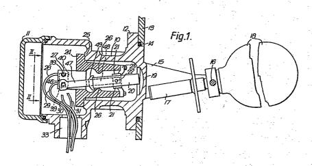
BESTOBELL MOBREY LIMITED GJE 5079/435 FLOAT OPERATED ELECTRICAL SWITCH ASSEMBLY.
