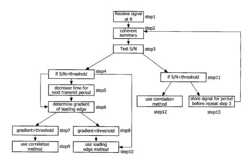
(57) Abstract: In a GPS or GSM system using DSSS signals, accurate and robust time-of-flight signal processing is achieved by selection of leading-edge or correlation techniques based on a variety of tests and environmental conditions.
