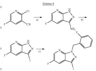
[a): hydrazine hydrate, 1,2-ethanediol; b): isopentyl nitrile, NaI, THF; b): 2-fluorobenzyl bromide, Cs<sub>2</sub>CO<sub>3</sub>, DMF;].
