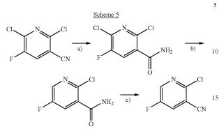
[a): sulphuric acid; b): zinc, methanol, glacial acetic acid; c): trifluoroacetic anhydride, dichloromethane].
