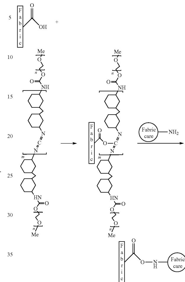
40 Since the efficiency of a reaction between a reactive residue in a fabric and a fabric care component is increased due to a carbodiimide-based compound, a reactive fabric care component bonded to the fabric may be not easily 45 detached during general washing with a detergent, a soap, or the like, but almost permanently attached to the fabric.
