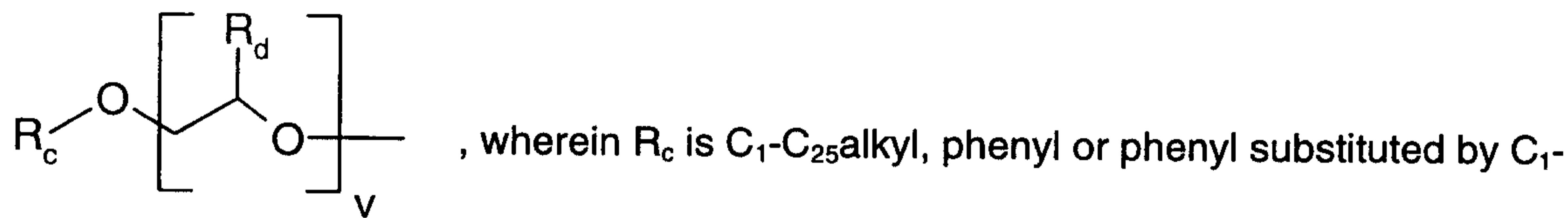
C<sub>18</sub>alkyl, R<sub>d</sub> is hydrogen or methyl and v is a number from 1 to 50. These monomers are for example derived from non ionic surfactants by acrylation of the corresponding alkoxylated alcohols or phenols. The repeating units may be derived from ethylene oxide, propylene oxide or mixtures of both.
