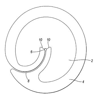
(57) Abstract: A wound dressing for post-operative sites requiring drainage, comprising a thin film or film/foam laminate layer with an adhesive applied to one surface thereof; an absorbent layer positioned on the adhesive surface of the thin film layer, the dressing being provided with an aperture to accommodate a drainage tube; and the dressing being slit from the aperture to an outer edge of the dressing.
