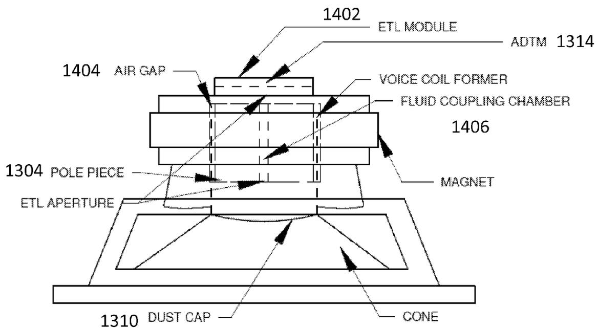
HF ETL MODULE COMMUNICATIVE WITH DRIVER THROUGH POLE PIECE AT THE DUST CAP
