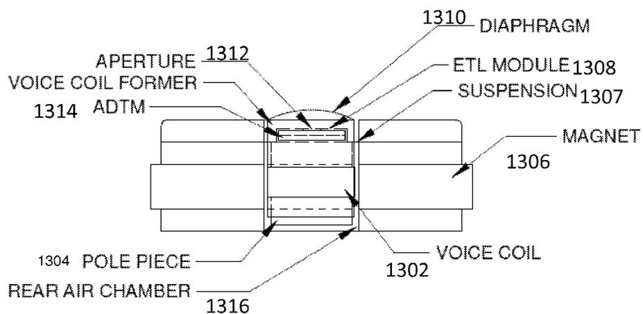
DOME TYPE DRIVER WITH THE ETL LOCATED WITHIN THE COIL DIAPHRAGM CHAMBER
