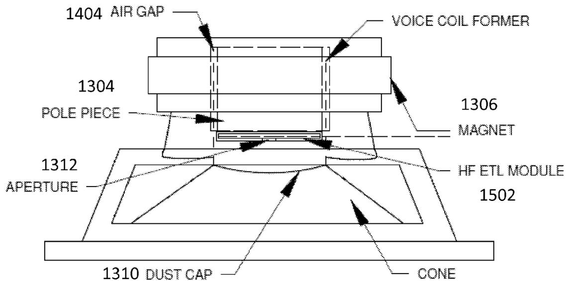
HF ETL MODULE RESTS ATOP POLE PIECE
