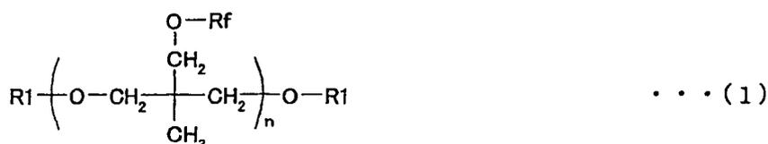
where Rf is selected from CH<sub>2</sub>CF<sub>3</sub> and CH<sub>2</sub>CF<sub>2</sub>CF<sub>3</sub>; n represents a value of 5 to 20; and each R1 represents a functional group capable of initiating an ultraviolet curing reaction and one of the two R1s in the structural formula (1) may be a hydrogen atom;
