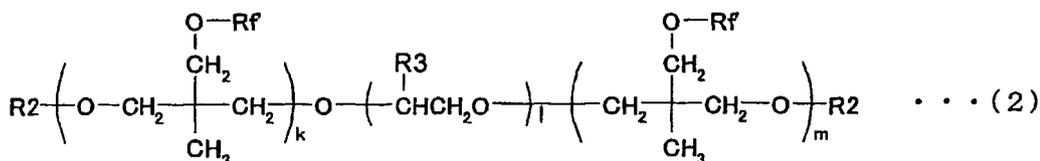
where Rf is selected from CH<sub>2</sub>CF<sub>3</sub> and CH<sub>2</sub>CF<sub>2</sub>CF<sub>3</sub>; l represents a value of 1 to 20; k and m each represent a value of 1 to 8; each R2 represents a functional group capable of initiating an ultraviolet curing reaction and one of the two R2s in the structural formula (2) may be a hydrogen atom; and R3 is selected from a hydrogen atom and a methyl group.
