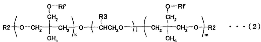
where Rf is selected from CH<sub>2</sub>CF<sub>3</sub> and CH<sub>2</sub>CF<sub>2</sub>CF<sub>3</sub>; l represents a value of 1 to 20; k and m each represent
