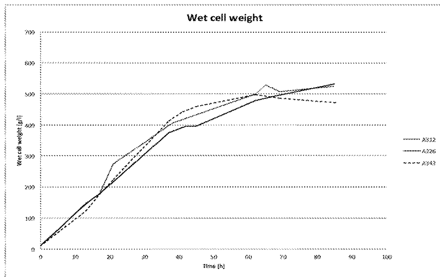
Figure 4: Cell growth profile indicating cellular growth similarity for 3 different mAb1 antibody strains A, B & C in 20L fermentors.
