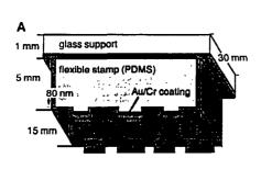
(57) Abstract: A method and apparatus for providing electric microcontact printing is provided. A stamp is brought into contact with the surface of a substrate to provide high resolution features. Aspects of the invention may be used for data storage, microcontact printing, and for other applications requiring high resolution pattern transfer.
