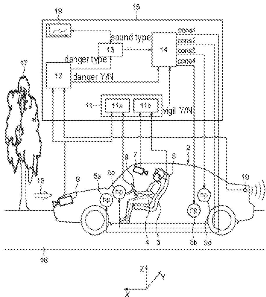
**DETECTION SYSTEM FOR A MOTOR VEHICLE, FOR INDICATING WITH THE AID OF A SOUND STAGE A LACK OF VIGILANCE ON THE PART OF THE DRIVER IN THE PRESENCE OF IMMEDIATE DANGER**
