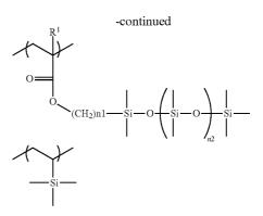
**[0093]** In the structure of the recurring unit having a functional group with a silicon atom, the definition and the preferred range of  $R^1$  are the same as those of  $R^1$  in the structure of the recurring unit having a functional group with a fluorine atom mentioned above.  $R^2$  represents an alkyl group having from 1 to 8 carbon atoms, n1 indicates an integer of from 1 to 5, and n2 indicates an integer of from 1 to 100.
