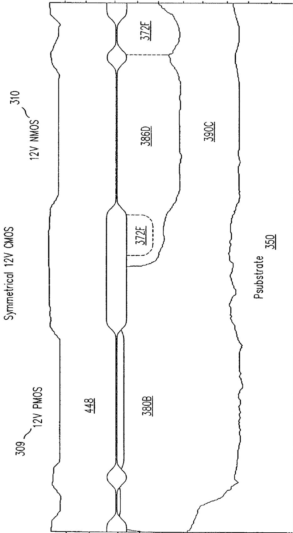
Threshold Adjust Implant-Second Stage
