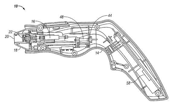
(57) Abstract: An RF device (10) has a support structure (18). An RF electrode (20), coupled to the support structure (18), includes conductive and dielectric portions. A cooling member (22), coupled to the support structure, is configured to cool a back surface of the RF electrode (20). The cooling member (22) is distanced from the back surface of the RF electrode (20).
