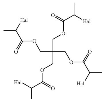
In the formulae above Hal represents chlorine or bromine. These initiator molecules are prepared by the reaction of a reactive functional derivative of  $\alpha$ -halogen carboxylic acid of the formula
