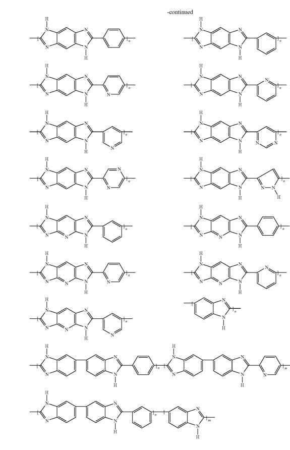
where n and m are each an integer greater than or equal to 10 is formed in step C).
