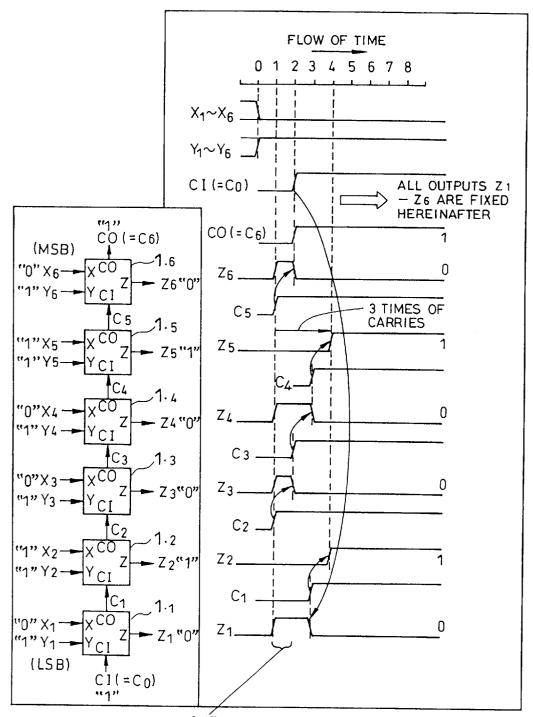
ZONE WHERE TEMPORARY VALUE OF OUTPUT Z IS OUTPUT IN THE CONDITION OF INPUTS X AND Y IRRESPECTIVE OF PRESENCE AND ABSENCE OF CARRY
