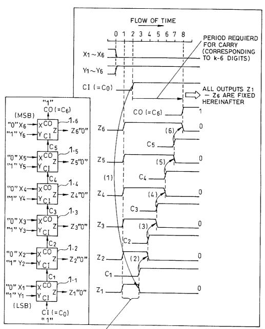
ZONE WHERE TEMPORARY VALUE OF OUTPUT Z IS OUTPUT IN THE CONDITION OF INPUTS X AND Y IRRESPECTIVE OF PRESENCE AND ABSENCE OF CARRY
