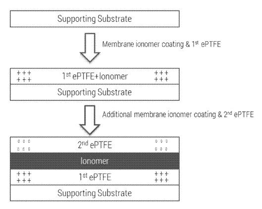
Double reinforced solid polymer electrolyte membrane
