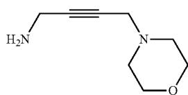
The first one may be received by reaction of propargyl amine with formaldehyde and morpholine, the second and third ones by reaction of propargyl alcohol with formaldehyde and piperidine or morpholine, respectively.
