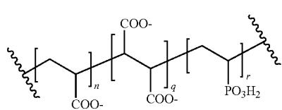
which is a terpolymer of acrylic acid, maleic acid and vinylphosphonic acid, wherein q and r are integers, the sum q+r corresponds to p in formula 1 and the ratio q/r is from 10:90 to 90:10, preferably 20:80 to 80:40, most preferably from 40:60 to 60:40.
