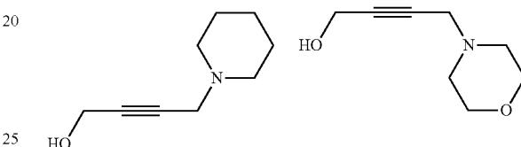
20 These may be received by reaction of propargyl alcohol with formaldehyde and piperidine or morpholine, respectively.
