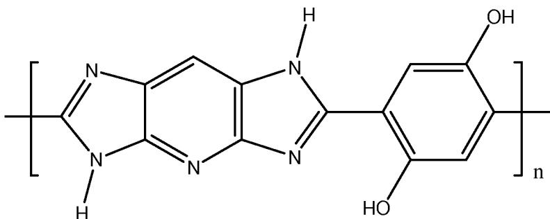
**[0028]** Polypyridobisimidazole fiber can be distinguished from the well known commercially available PBI fiber or polybenzimidazole fiber in that that polybenzimidazole fiber is a polybibenzimidazole. Polybibenzimidazole fiber is not a rigid rod polymer and has low fiber strength and low tensile modulus when compared to polypyridobisimidazoles.
