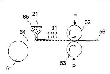
(57) Abstract: A method for a binder-free manufacturing a nanostructured porous film, e.g. for use in solar cells, comprises the steps of: preparing a suspension of semi-conducting nanometer-sized particles in a volatile suspending agent (21), depositing the particle suspension on a conducting substrate, removing the suspending agent by evaporation (31), and compressing (P) the deposited particles for mechanical and electrical interconnection.
