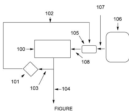
(57) Abstract: Industrial fluids can be monitored by employing differential ion mobility spectrometer to sample the industrial fluids. This process may also include controlling an industrial device or an industrial process using the results of the output from the field asymmetric ion mobility spectrometer. The process may also include employing a device to condition the sample prior to introducing the sample into field asymmetric ion mobility spectrometer.
