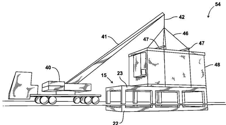
a lifting device that lifts each from the transport vehicle to the site.
