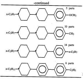
The first and second components in the above composition belong to the component [B] of the present invention; the succeeding 4 components belong to the component [C] of the present invention; and the remaining 6 components belong to the component [D] of the present invention. The specific features of this nematic liquid crystal composition are shown in Table 1.
