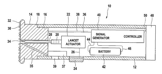
(57) Abstract: A lancing device (10) where electrical stimulation is applied to a skin sampling site prior to making an incision to achieve at least one of pain masking and bodily fluid engorgement at the site. The electrical stimulation is supplied by a low current high voltage AC signal generator (40) in sufficient quantities to produce vasodialation and/or pain masking.
