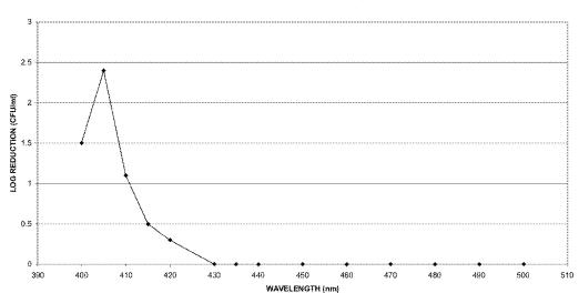
Log Reduction v Wavelength for S.aureus 4135 (2 hour exposure at 5cm distance) \* Filter transmission -50% (3.27mW average power)
