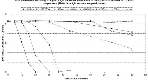
Effect of different wavelength ranges of light on the inactivation rate of Staphylococcus aureus NCTC 4135 suspensions (100%; 5cm light source - sample distance)
