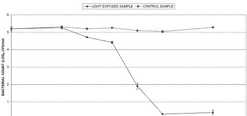
Streptococcus pyogenes inactivation by treatment with 405 nm LED array
