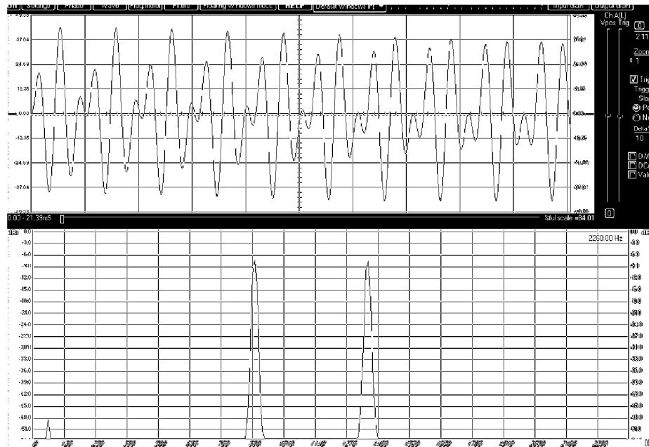
Figure 39a Mixer Test; Sine Waves (No Flame): 900 Hz (-7 dB); 1,300 Hz (-7 dB)
