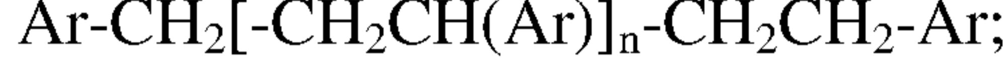
wherein each Ar is a phenyl group, for each molecule in the distribution, "n" is a whole number in the range of 0 to 6, and wherein the distribution is characterized by a majority of the molecules in the distribution having an "n" value of 0 and a minority, not exceeding 49 GPC area%, of the molecules in the distribution having an "n" value of 1, 2, 3, 4, 5 or 6 wherein the GPC area% for "n" equals 1 > "n" equals 2 > "n" equals 3 > "n" equals 4 > "n" equals 5 > "n" equals 6;
