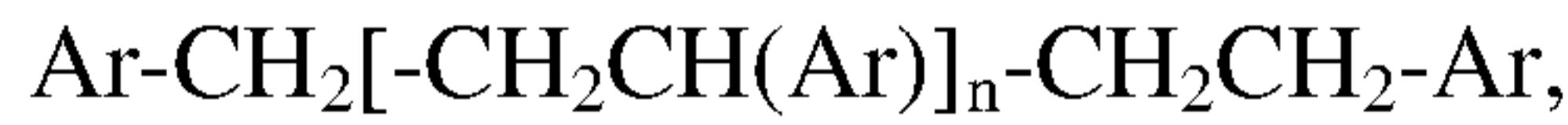
wherein each Ar is a phenyl group, and, for each molecule in the distribution, "n" is a whole number in the range of 0 to 6 and wherein the distribution includes molecules having "n" values from 1 to 6.
