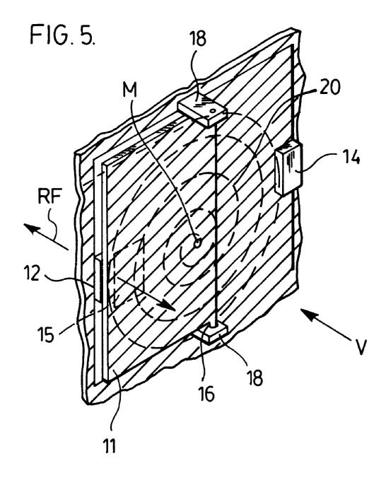
This invention relates to a display element and to an array thereof, wherein a disk mounting a permanent magnet may be electromagnetically driven by magnetic field forming members between ON and OFF positions in which positions, opposite disk surfaces of contrasting appearance are displayed in a viewing direction.
