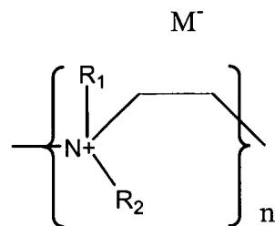
and salts and copolymers thereof, where n is a positive integer and y and z are integers of one or more, and R, R<sub>1</sub>, R<sub>2</sub> and R<sub>3</sub>, independently, is H or a substituted or unsubstituted alkyl, alkylamino or aryl group.
