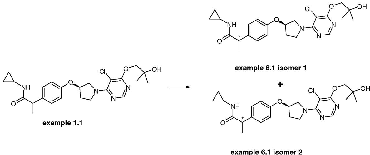
The stereoisomers of example 1.1 are separated by prep. chiral HPLC.
