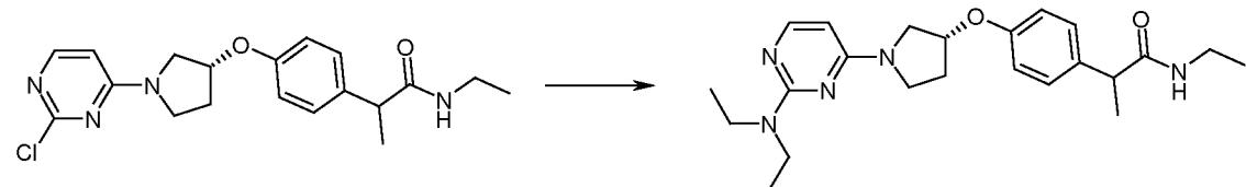
50 mg (0.13 mmol) of example XII, 40  $\mu$ l (0.38 mmol) of diethylamine and 30  $\mu$ l (0.17 mmol) of DIPEA are dissolved in 2 ml ACN. The reaction mixture is stirred at 110 °C
