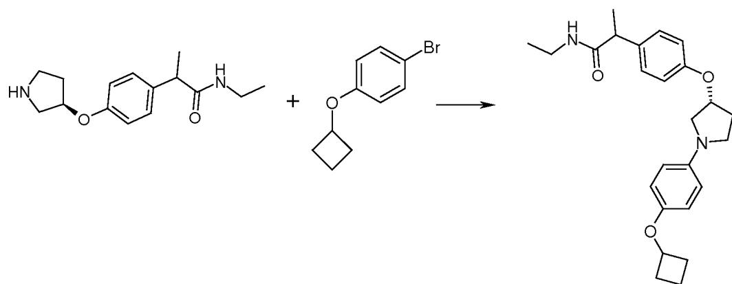
To 30 mg (0.10 mmol) of example III, 27 mg (0.12 mmol) of 1-bromo-4-cyclobutoxybenzene and 40 mg (0.40 mmol) of sodium tert. butoxide in 2 mL Dioxan are added under inert atmosphere 10 mg (0.01mmol) of chloro(2-dicyclohexylphosphino-
