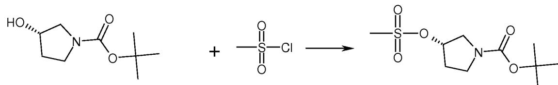
20 To 3.44 g (187 mmol) (S)-1-Boc-3-pyrrolidinol in 15 mL THF are added 1.70 mL (21.6 mmol) of methanesulfonyl chloride at 0°C. The reaction mixture is stirred for 1h. Water is added and it is extracted with EtOAc (3x). The organic layer is washed with an aq. NaHCO<sub>3</sub> solution and dried over MgSO<sub>4</sub>. The solvent is removed in vacuo.
