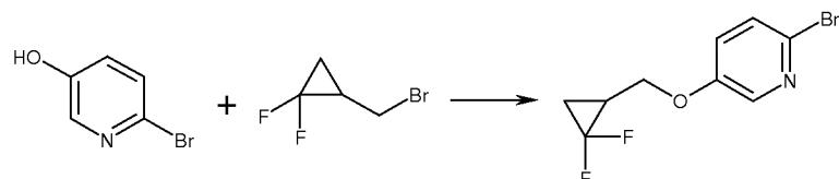
The mixture of 5.00 g (28.7 mmol) of 2-bromo-5-hydroxypyridine, 6.14 g (35.9 mmol) 15 of 1-bromomethyl-2,2-difluorocyclopropane and 9.93 g (71.8 mmol) of K<sub>2</sub>CO<sub>3</sub> in 100 ml ACN is stirred at 70 °C for 14 h. The reaction mixture is diluted with EtOAc, washed with water and 1N aq. NaOH, dried over MgSO<sub>4</sub>, filtered and the solvent is removed in vacuo.
