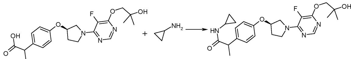
To 42 mg (0.10 mmol) of example XIII in 3 mL DMF are added 42  $\mu$ l (0.30 mmol) of 10 TEA and 32 mg (100  $\mu$ mol) TBTU and it is stirred at r.t. for 10 min. Then 14  $\mu$ l (0.20 mmol) of cyclopropylamine are added and the resulting mixture is stirred at r.t over night. The mixture is directly purified by prep. HPLC-MS (ACN/H<sub>2</sub>O/NH<sub>4</sub>OH).
