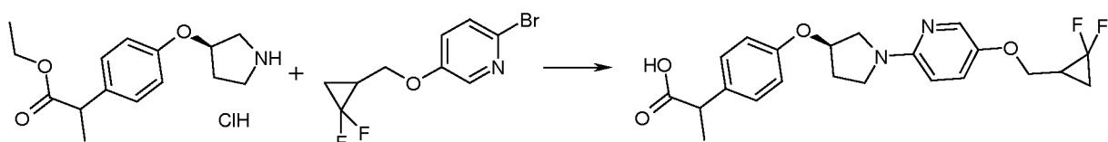
1.40 g (4.67 mmol) of example V are dissolved in 30 ml dioxane under nitrogen atmosphere. 1.20 g (12.1 mmol) of sodium tert.butylate and 0.80 g (3.0 mmol) of
