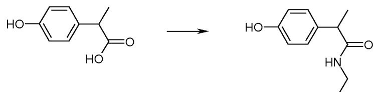
To 4.00 g (24.1 mmol) 2-(4-hydroxyphenyl)propionic acid in 50 mL THF and 5 mL DMF are added 6.76 g (66.1 mmol) TEA and 8.50 g TBTU. The reaction mixture is stirred at r.t. for 5 min, then 36.1 mL (2 mol/l solution; 72.2 mmol) ethylamine are 10 added. The reaction mixture is stirred at r.t. 5 h. The solvent is removed in vacuo and the crude product is purified by prep. HPLC-MS (ACN/H<sub>2</sub>O/NH<sub>4</sub>OH).
