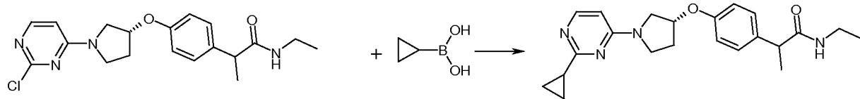
Under inert atmosphere 50 mg (0.13 mmol) of XII are dissolved in 3 ml dioxane. 30 mg (0.35 mmol) of cyclopropylboronic acid, 55 mg (0.26 mmol) of  $K_3PO_4$  and 5 mg (0.01 mmol) of 1,1'-bis (diphenylphosphino)ferrocene dichloropalladium(II) are added. The reaction mixture is stirred at 90 °C over night. The same amounts of the boronic acid, the base and of the catalyst are added. The reaction mixture is stirred at 120 °C in a microwave oven for 5 h and at 100 °C over night. The reaction mixture
