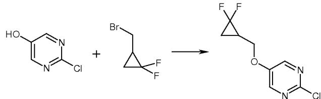
The mixture of 150 mg (1.15 mmol) of 2-chloro-5-hydroxypyrimidine, 295 mg (1.72 mmol) of 1-bromoethyl-2,2-difluorocyclopropane and 318 mg (2.30 mmol) of  $K_2CO_3$  in 3 ml DMF is stirred at 80 °C over night. The reaction mixture is extracted with water and DCM. The organic layer is dried, filtered and the solvent is removed in vacuo. The residue is purified by prep. HPLC-MS (MeOH/H<sub>2</sub>O/NH<sub>4</sub>OH).
