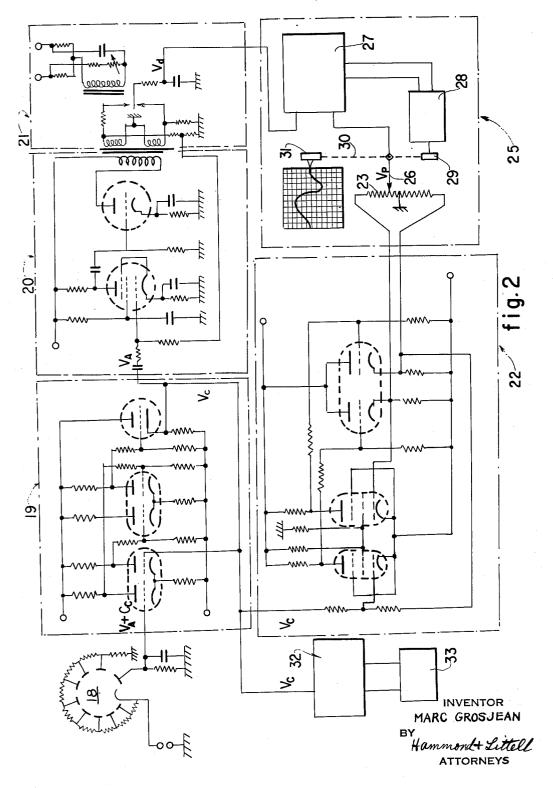
REGISTERING APPARATUS FOR MEASURING CIRCULAR DICHROISM
