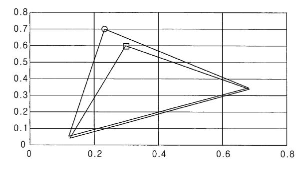
□LCD ASSEMBLY O: NTSC STANDARD
