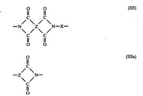
in which Z is the tetravalent radical of an aromatic tetracarboxylic acid onto which in each case two carbonyl groups are bonded in the ortho- or periposition, Z' is the trivalent radical of an aromatic aminocarboxylic acid onto which two carbonyl groups are bonded in the ortho- or periposition and X is the divalent radical of an organic diamine.
