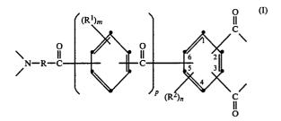
in which  $R^1$  and  $R^2$  are halogen, nitro, aryl, aryloxy, alkyl or alkoxy, m is 0 or a number from 1 to 4, n is 0 or a number from 1 to 3 and p is 0, 1 or 2, the free carbonyl groups are bonded in the ortho-position relative to one another and R is a divalent aromatic radical which is substituted by at least one alkyl group or aralkyl group, are autophotocrosslinkable. They are suitable for the production of protective films and photographic relief images.
