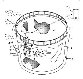
hand-held device (9) of an operator, and wherein the flow rate of the injected oxygen is controlled such that the measured current concentration of dissolved oxygen approaches a pre-defined reference value.
