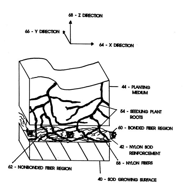
EXPLODED VIEW OF ROOT PENETRATION IN PATTERN BONDED NYLON SPUNBOND FABRIC
