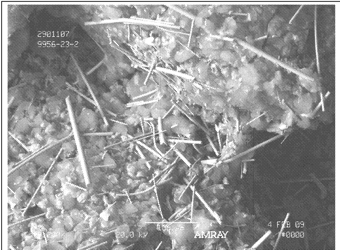
Figure 3: Scanning electron micrograph of an aerogel - mineral fibre composite made with high pH water.
