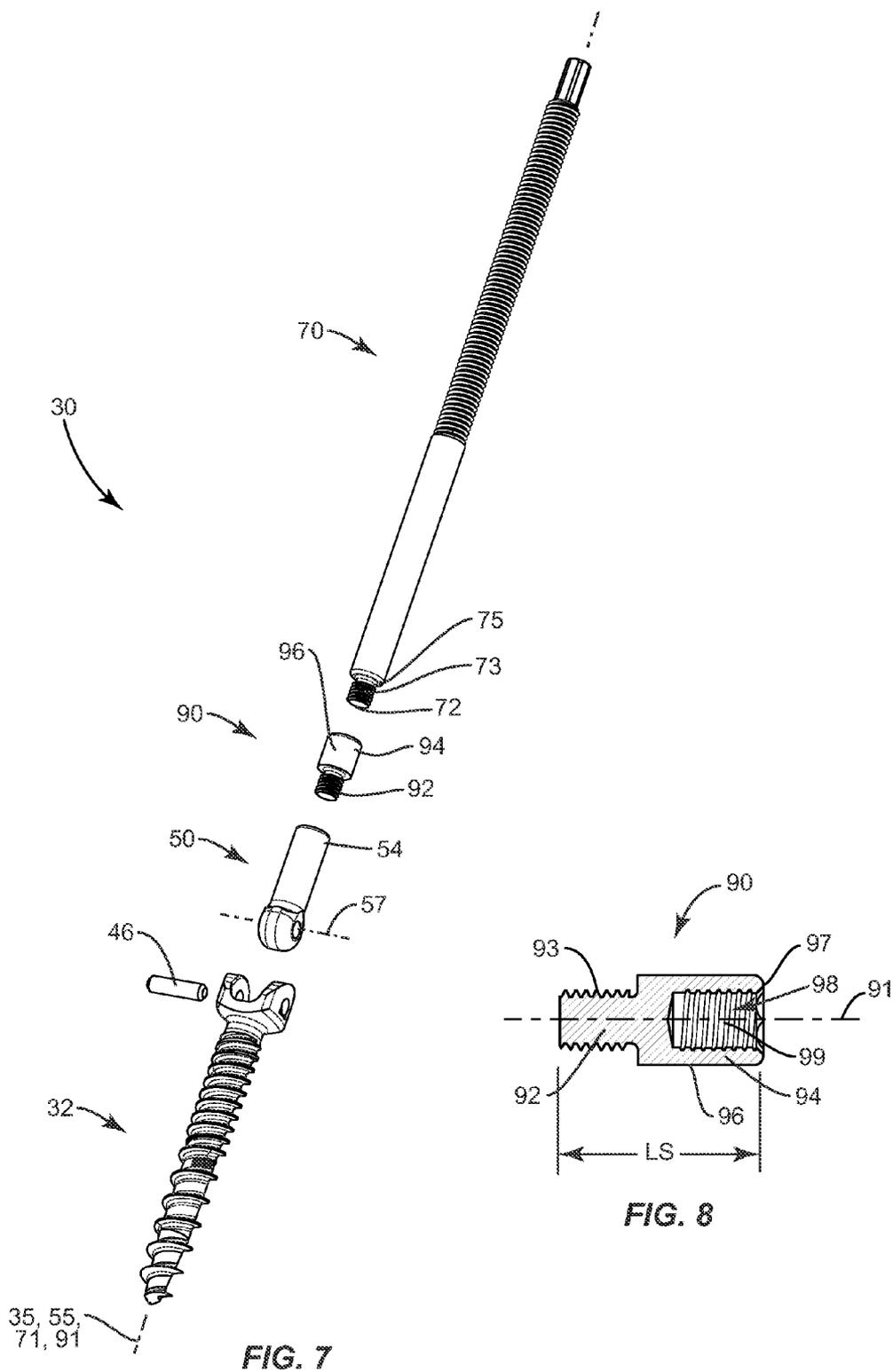
**MODULAR PIVOTABLE SCREW ASSEMBLY AND METHOD**
