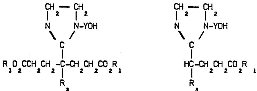
The imidazolines can be prepared from a variety of acids ranging from  $\text{C}_4$  -  $\text{C}_{22}$ . They may be normal straight chain fatty acids or acids with additional groups such as hydroxy. They may also be alkylaryl or alkylcyclo aliphatic acids.
