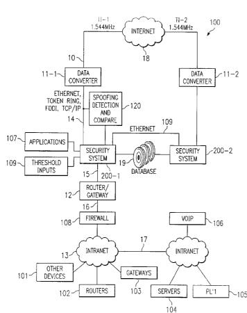
(57) Abstract: A traffic management system sniffs data arriving at any point in a system. The sniffer operates to extract certain data from each address. This data could be, for example, the IP address data and the physical address data. The extracted data is then used to access different data bases to determine if matches occur. Time stamps, sequencing and other parameters of each piece of data entering a system are used to control data access.
