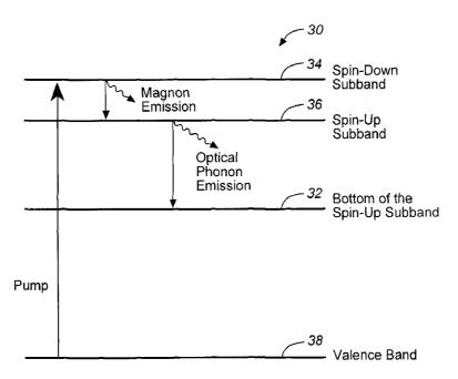
(57) **Abstract:** A method of THz photon generation comprising: providing a magnon gain medium; wherein the magnon gain medium supports generation of nonequilibrium magnons; and injecting nonequilibrium electrons into the magnon gain medium. Propagation of nonequilibrium electrons in the magnon gain medium causes generation of nonequilibrium magnons. Interaction between nonequilibrium magnons causes generation of THz photons.
