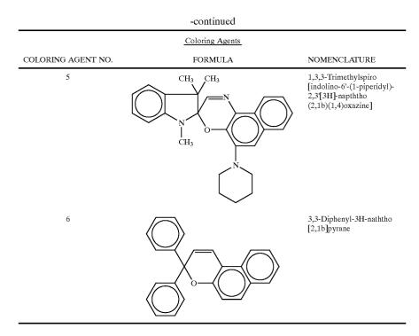
In the photochromic materials or glasses obtained, the <sup>30</sup> times of half-darkening and half-lightening are measured. The light source is a mercury vapor lamp, and the measurement of transmission is done at the wavelength of  $\lambda_{max}$  of the coloring agent and at room temperature on a 2-mm-thick sample. Table II below recapitulates the results obtained for <sup>35</sup> various photochromic materials according to the invention.
