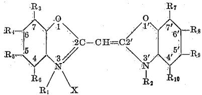
wherein R<sub>1</sub> and R<sub>2</sub> are alkyl or oxyalkyl groups, and R<sub>3</sub> to R<sub>10</sub> may be hydrogen atoms, or any of them may represent substituted groups such as alkyl, alkoxy, amino and substituted amino groups, or halogen atoms, and X is an acid radical, which compound is colourless in ethyl alcoholic solution. By the term "colourless in ethyl alcoholic solution" is meant that a solution of the compound in ethyl alcohol has an absorption maximum not greater than 4000 Å.
