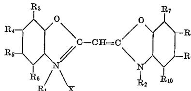
where R<sub>1</sub> and R<sub>2</sub> are selected from the class consisting of alkyl and oxyalkyl groups and R<sub>3</sub> to R<sub>10</sub> inclusive are selected from the class consisting of hydrogen atoms, halogen atoms and alkyl, alkoxy, amino and substituted amino groups, and X is an acid radicle, which compound is colourless in ethyl alcoholic solution.
