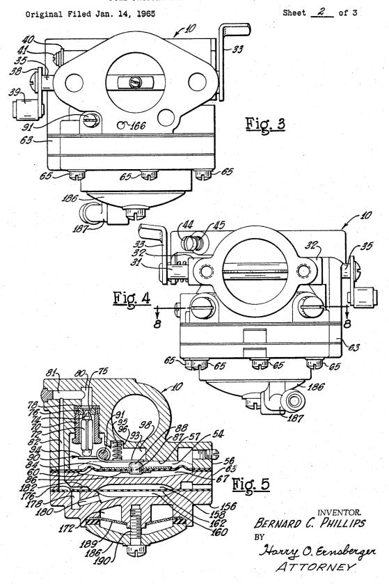
FUEL FEEDING AND CHARGE FORMING APPARATUS
