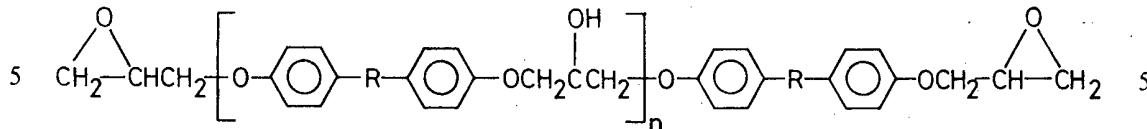
where  $n$  is an integer from 0—42 and R is an alkylene group of 1—4 carbon atoms. The epoxy resins utilized in the present invention contain at least two epoxy groups per molecule and therefore, upon curing of the composition, introduce no uncross-linkable extractable portions into the coating.
